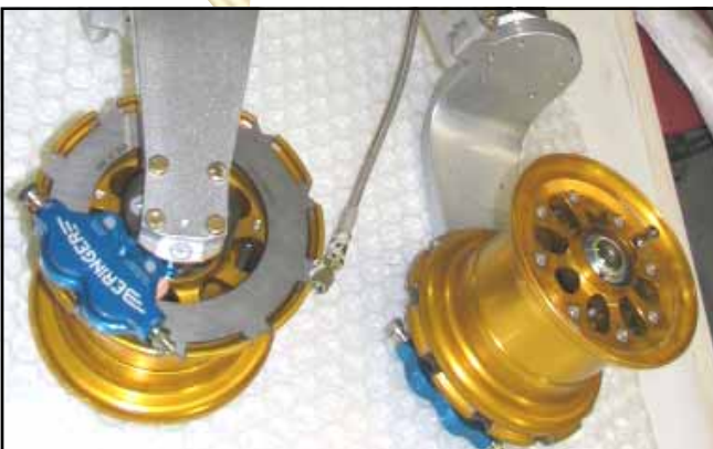
BERINGER Wheels and brakes mounted on Race GLASAIR III landing gear
