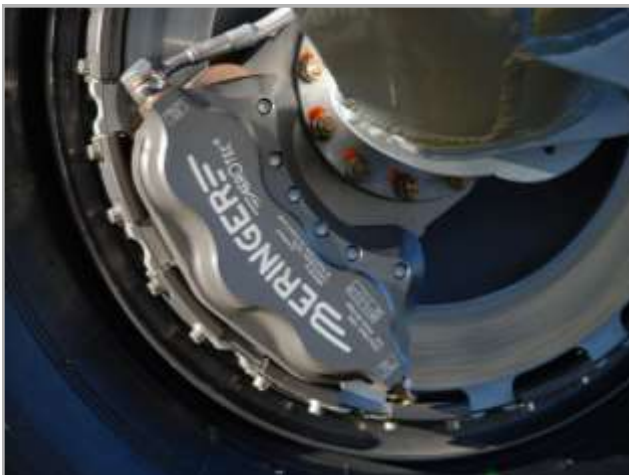
Wheel & brake set for Pilatus PC-6
